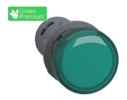
Easy Harmony XA2E, Monolithic pilot light, plastic, green, Ø22, integral LED, screw clamp terminals, 220 V DC
